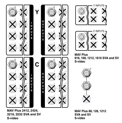
Figure 2-14 — MAV Plus S-video connections
